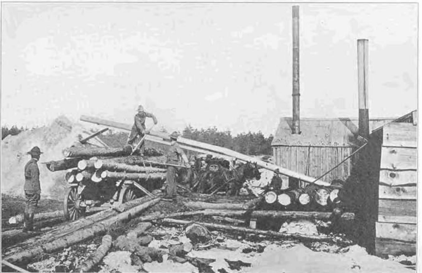
UNLOADING SMALL LOGS AT AN AMEX MILL IN CENTRAL FRANCE. NOTE THE SPOUT THROUGH WHICH THE SAWDUST IS BLOWN TO LARGE SAWDUST PILE AT THE LEFT
