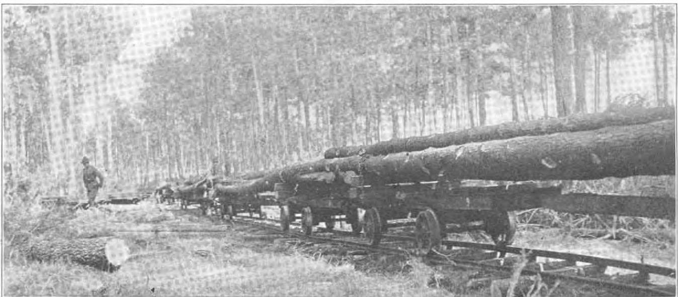
LONG MARTIME PILING LOADED ON AMERICAN NARROW GAUGE CARS READY FOR TRANSPORTATION FROM THE FOREST TO THE MAIN LINE RAILWAY SHIPPING POINT NEAR PONTENX, LANDES, FRANCE
